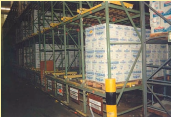
Flow racks with full width rollers and brake rollers
