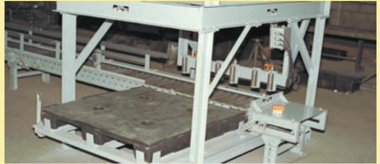
Low volume scissor lift type palletizing of containers
