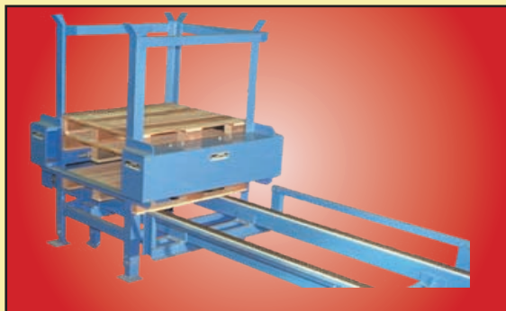
Pallet dispenser feeding chain conveyors.
