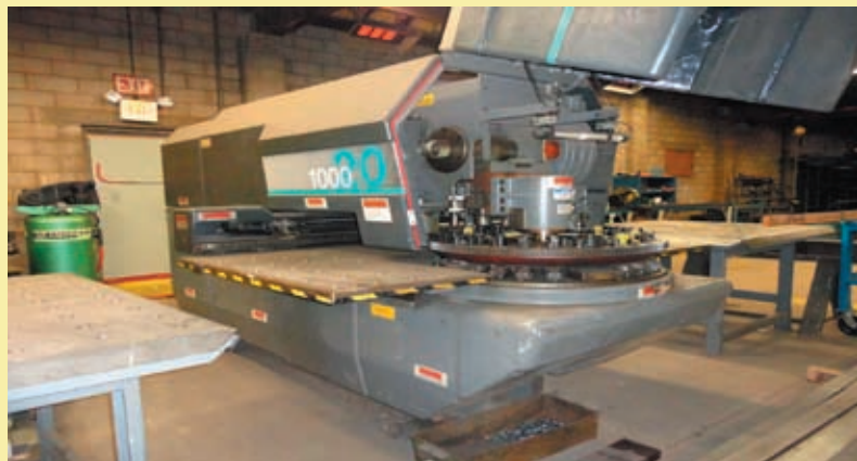
Up to 1/4" thick material can be punched efficiently and accurately with our computer controlled turret multi-punch press.
