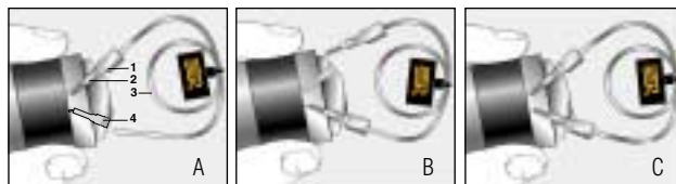
Fig. 1. Cut-away view of stainless steel sample loop installation.
