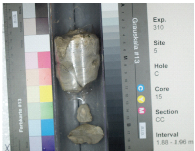
Figure 4. Example of core catcher samples from IODP 310. Core 5C-15CC, 85 mbsl, 26 mbsl. Note lamination.
