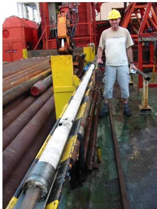
Figure 3. A continuous 3 m core of fossil reef material recovered as a single piece during IODP Expedition 310.
