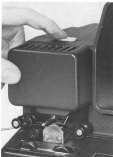
By rotation of the sprocket **8** you can inch the film forward and backward frame by frame.
