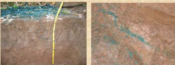
Figure 3. Preferential flow of Erioglaucine through macropores - (0.5-5 cm thickness) - created from shrinking of clay minerals
