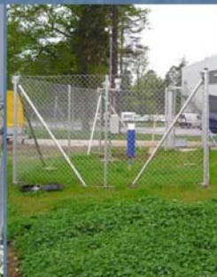
Meteorologic station (Prec., Temp., rel. Hum., Radiation, wind velocity)
