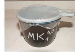
Fot. 2. The plastic cup with soil sample closed by PARAFILM M in the laboratory experiment (2001).
