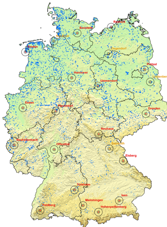
Figure 2: Site of installed wind turbines (blue points) in Germany and DWD weather radar (red points) and wind profiler (yellow points) sites surrounded by grey circles which represent the 5 km exclusion and the 15 km protection zones (with use of data of © Bundesamt für Kartographie und Geodäsie (2013), Frankfurt am Main).
