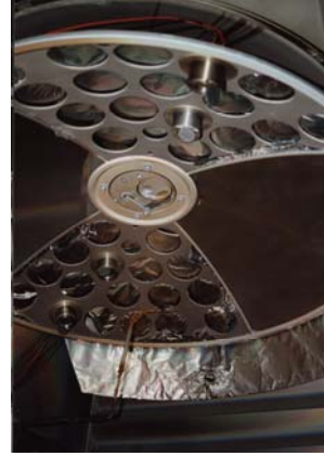
Fig. 8: Faraday Cup arrangement in the plant with MIEDA sensors placed instead of substrates at the substrate calotte
