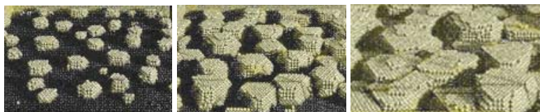
Fig. 2. Film growth: Nucleation – Coalescence – Continuous film (Floro et al. 2001)
