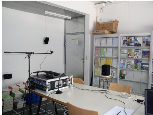
Illustration 1: test structure for environmental microphone test IEEG140, Inffeldgasse 16. In the picture: RME FireFace 800 Wandler, Mikrofone MIC1-MIC5, YAMAHA Monitor speakers, laptop for recording control
