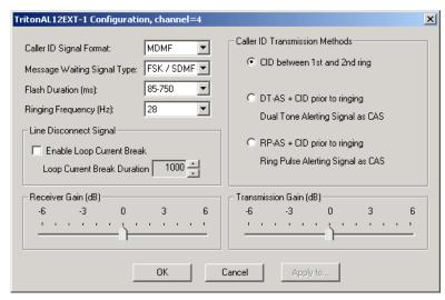
Figure 4. Triton Analog Trunk Properties window
