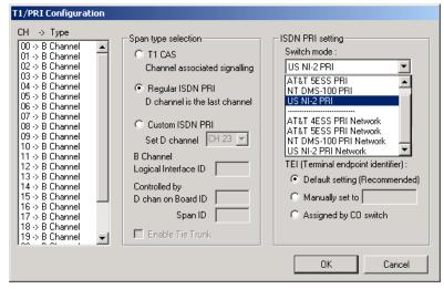
Figure 17. ISDN PRI Switch Mode
