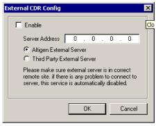
Figure 12. Enable external call data logging
