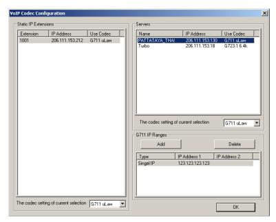
Figure 4. VoIP Codec Configuration window
