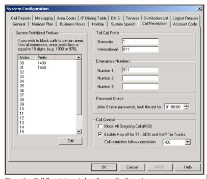
Figure 6. Call Restriction window, System Configuration
