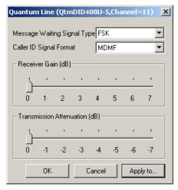
Figure 7. Quantum Line Properties dialog box for extensions
