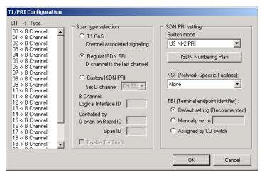
Figure 16. T1/PRI Configuration window
