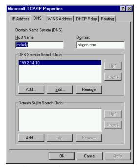
Figure 3. DNS Configuration window
