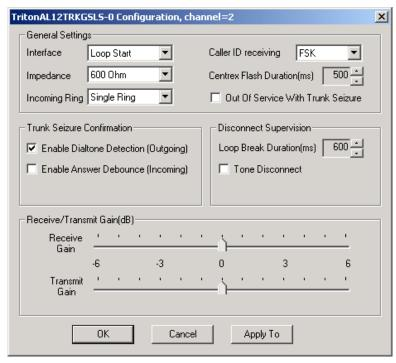
Figure 5. Triton Analog GSLS Trunk Properties window
