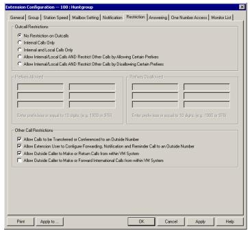
Figure 15. Restriction window, Extension Configuration
