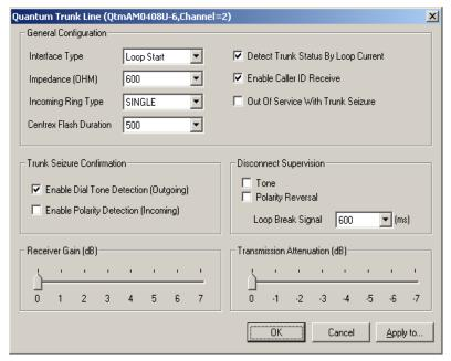
Figure 3. Quantum Trunk Line Properties window
