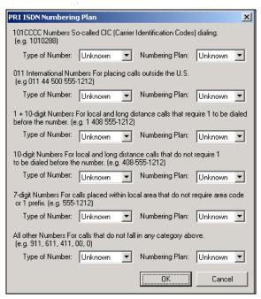
Figure 18. PRI ISDN Numbering Plan dialog box
