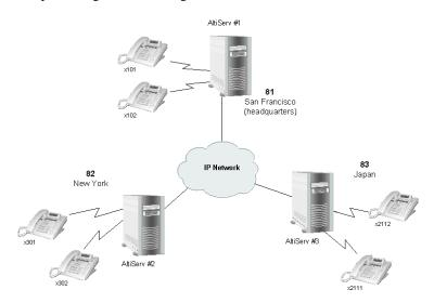
Figure 11. AltiServ-to-AltiServ Connection
