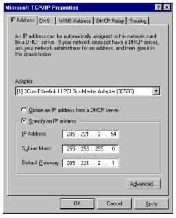
Figure 2. TCP/IP Configuration
