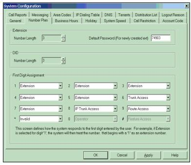
Figure 2. Number Plan window, System Configuration
