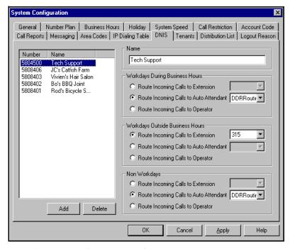
Figure 17. DNIS window, System Configuration
