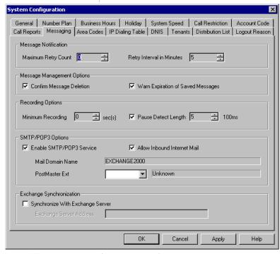
Figure 14. Messaging window, System Configuration
