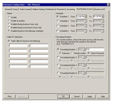
Figure 19. One Number Access window, Extension Configuration
