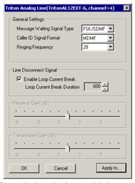
Figure 8. Triton Analog Station Line Properties dialog box
