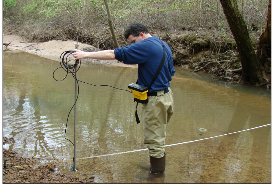
Figure 3. Velocity is often measured using a current meter (Ledbetter Creek, Calloway County, Kentucky).
