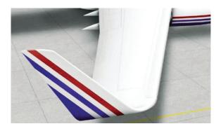
Figure 2: Blended winglet configuration [6]
