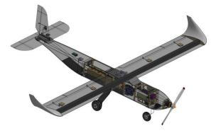
Figure 3: Isometric view of the model airplane with blended winglets [8]
