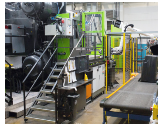
Waste container production on an ENGEL duo 4000: recyclate from post-consumer collections is processed.
