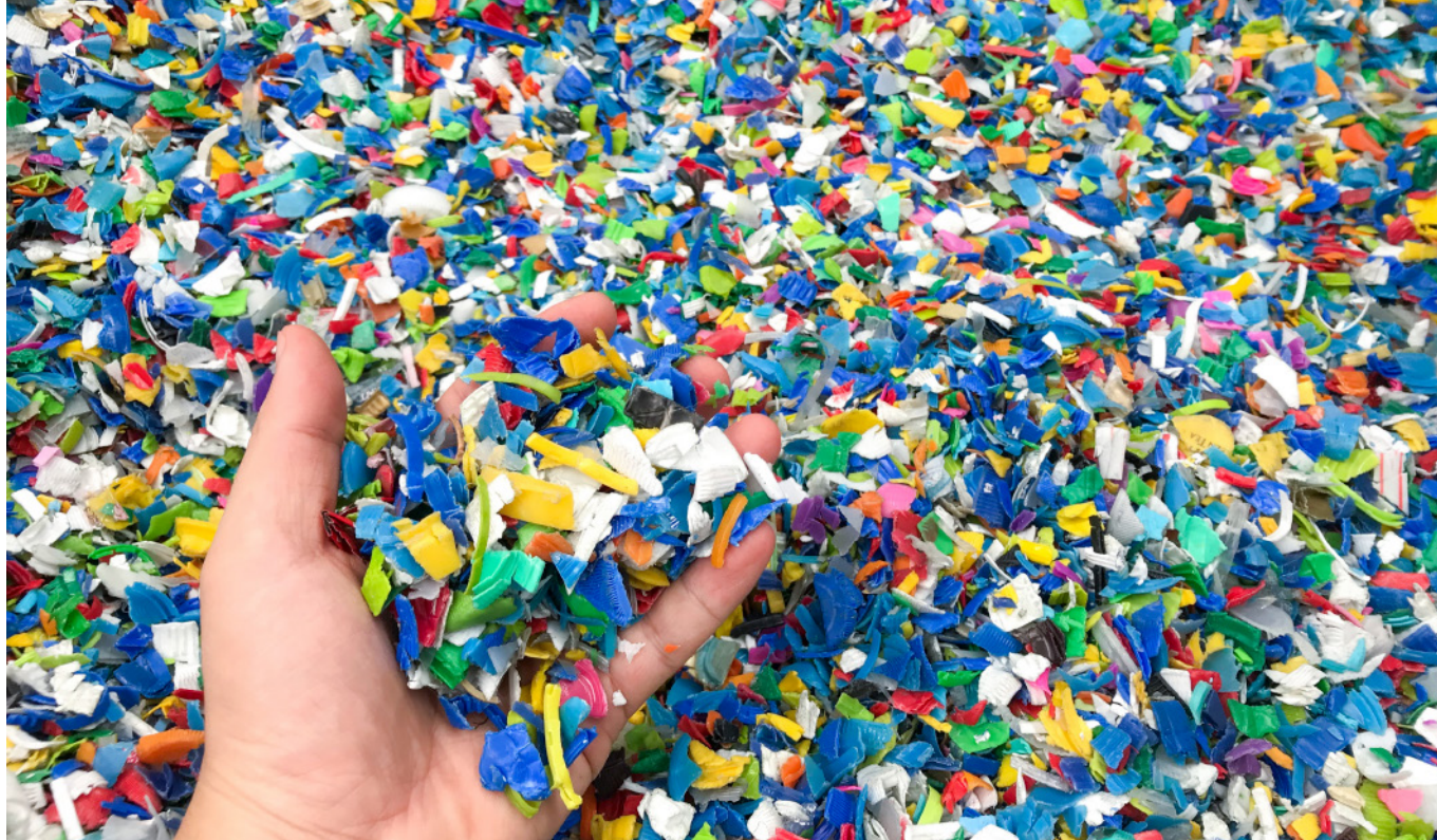
The aim of the innovation is to process plastic flakes, for example from post-consumer collections, directly in injection moulding without granulation.
