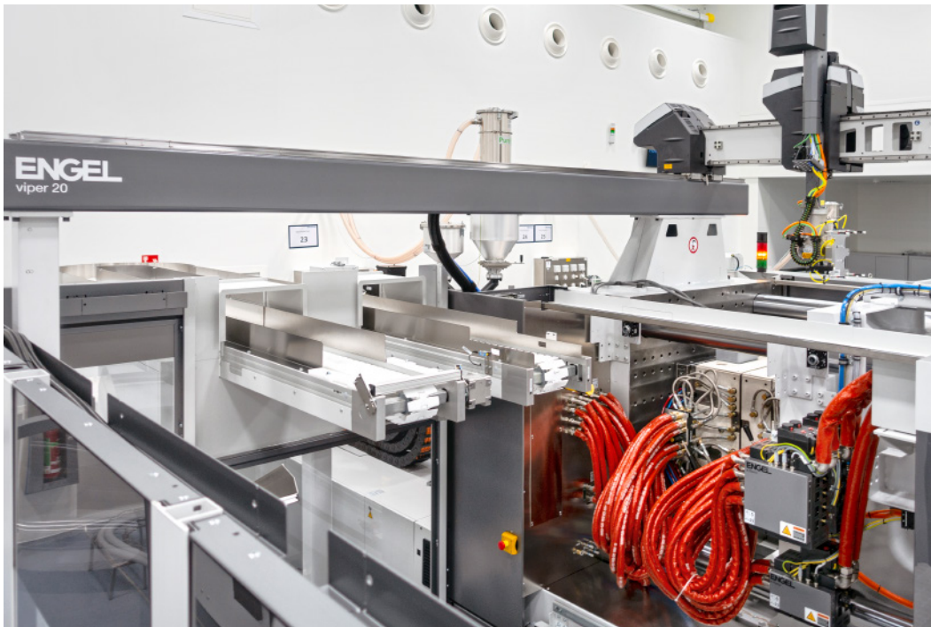
The viper 20 robots perform two tasks: demoulding the injection moulded parts from the mould and transferring the parts from the post-cooling area to the take out conveyor.
