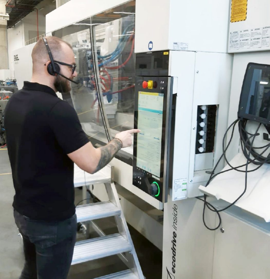
The bearing brackets are produced in the MuCell foam injection moulding process on an ENGEL e-victory 400 injection moulding machine.
