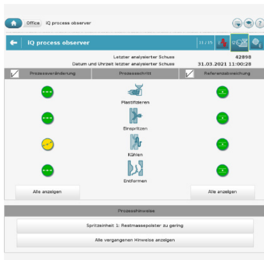
Figure 1: The overview page of the iQ process observer summarises all information about the current process status.
