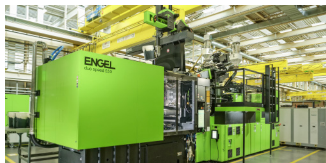
ENGEL's compact two-platen technology is one of the factors contributing to the high level of efficiency.
