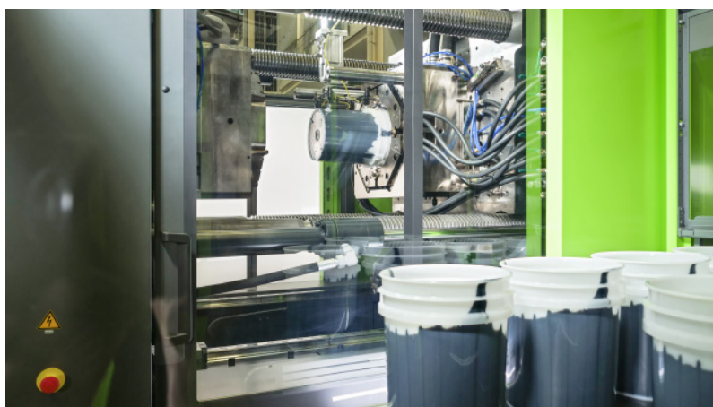
To demonstrate the high recycled content, a transparent skin material made of virgin material is combined with a black recycled material.
