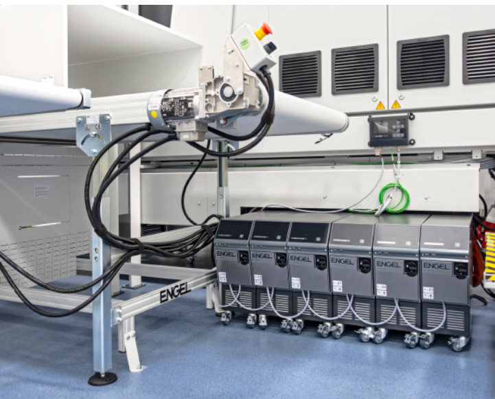
The use of e-temp temperature control units significantly increases the energy efficiency of the temperature control processes. Connected to the CC300 machine control via OPC UA, the temperature control units adjust their pump speed to the demand.
