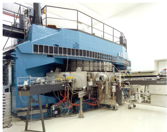
Figure 1: The isochronous cyclotron JULIC.
