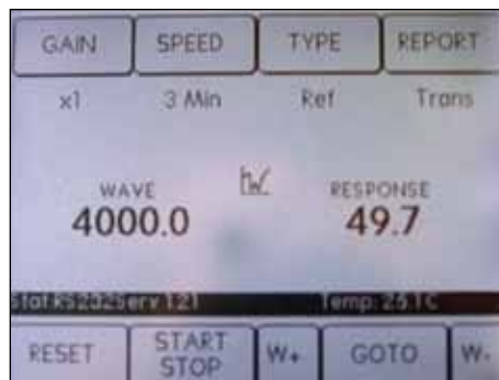
Set all instrument parameters and view spectra with the touch-screen display
