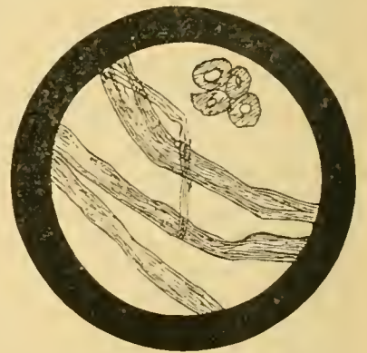
SPECIMENS OF JUTE FIBRES, MAGNIFIED, Showing also Cross Sections.
