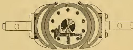
End View of Cylinder and Presser Beds.
