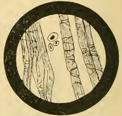
SPECIMENS OF HEMP FIBRES, MAGNIFIED, Showing also Cross Sections.
