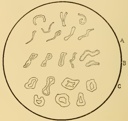
SECTIONS OF COTTON FIBRES MAGNIFIED.
