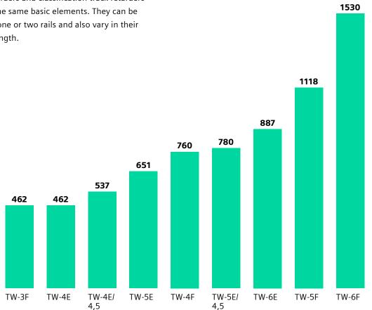
Retarding energy in kJ for an axle with an axle load of 22.5 t for single-rail or two-rail Trackguard Retarder TW-F and TW-E clasp retarders
