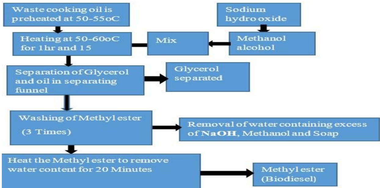
Figure 2 Conceptual flow chart of overall biodiesel production from waste cooking oil
