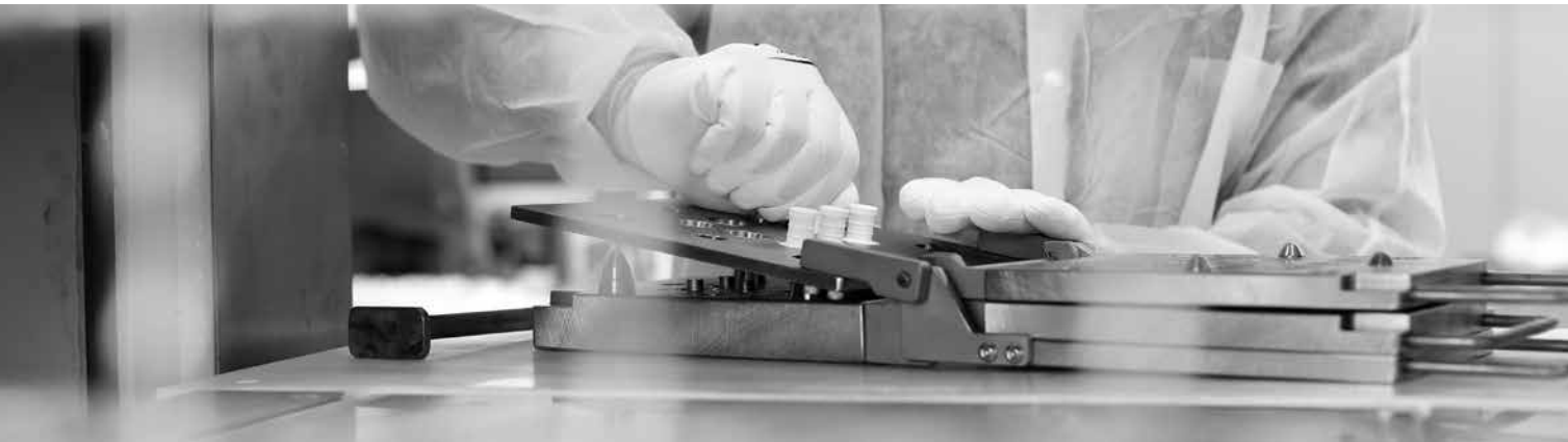
The small parts of the TRACOE silcosoft tubes are made in the silicone press
