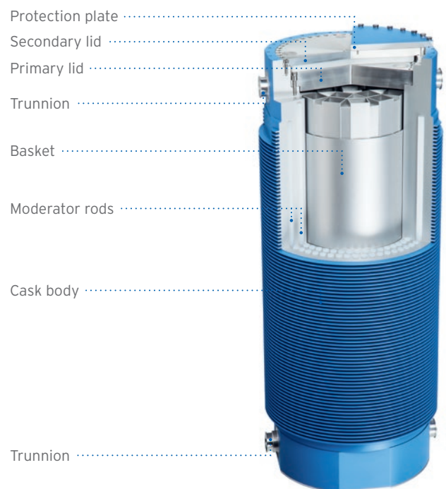
Figure 4: CASTOR® cask in storage configuration (example: CASTOR® V/19)
