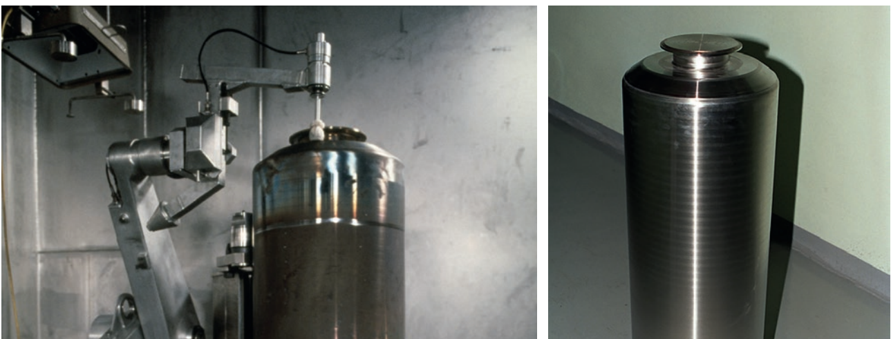
Figure 14: Loading of a cask with HAW canisters (left), single canister (right)
