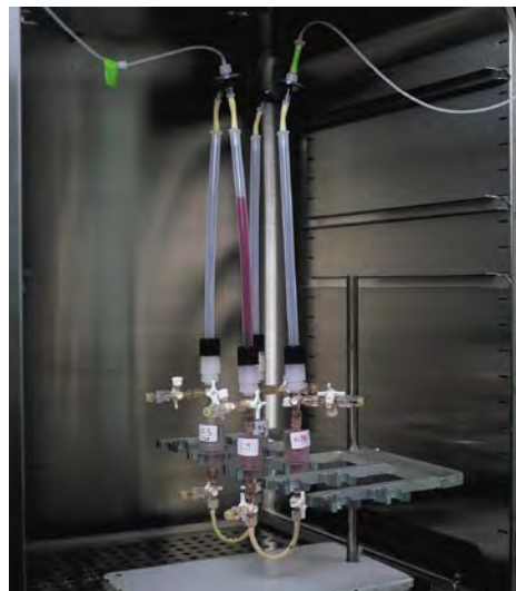
Fig. 1: Bioreactor system for seeding and 3D culture of cells into porous scaffolds under controlled perfusion. Controlled regimes of fluid flow are necessary to uniformly distribute cells in the scaffold and to maintain their viability and function even in the innermost pores (Wendt et al., 2003).
