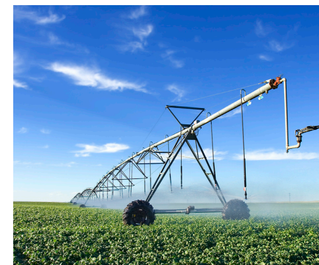
M6 With this overhead irrigation system it is possible to irrigate a circular area.
