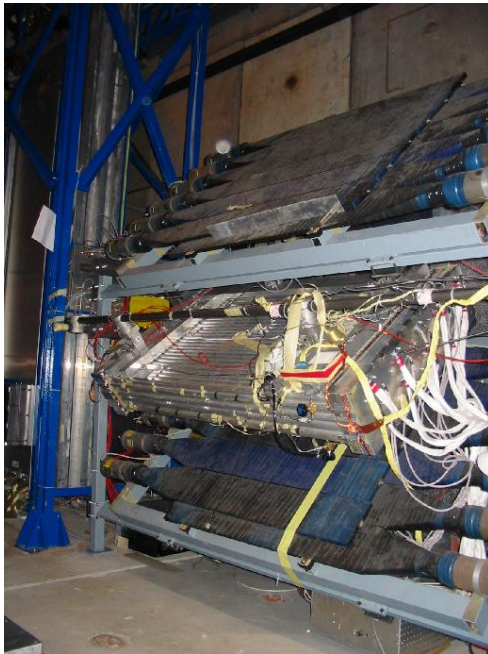
Figure 3.13: Layout and mechanical setup during period 'Age2'. MDT wires and hodoscope scintillator strips were parallel to each other. Only 2/3 of the MDT chamber was within the trigger acceptance; the pulse height could therefore only be monitored for the first 105 cm, measured from the MDT readout side.
