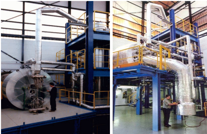
emergency and containment cooler tests at Forschungszentrum Jülich
