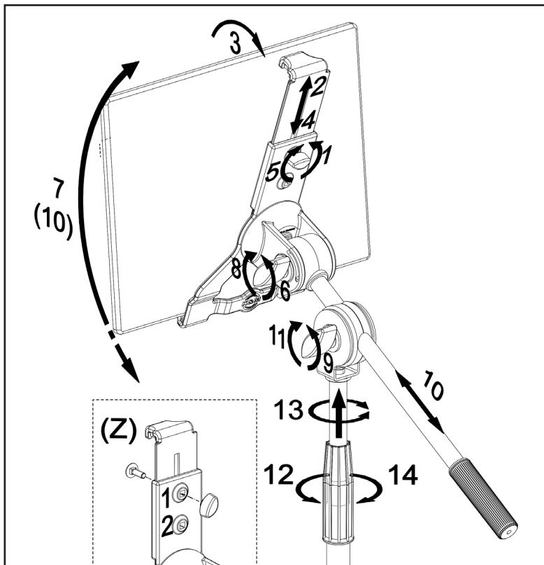
Open the lock nut at the slider 1 and pull the slider upward 2. Set the tablet on the lower holder arms and place it in the tablet holder 3. Make sure the back of the tablet lies flat against the holder. Set the slider on the tablet 4 and hand-tighten the lock nut 5.
