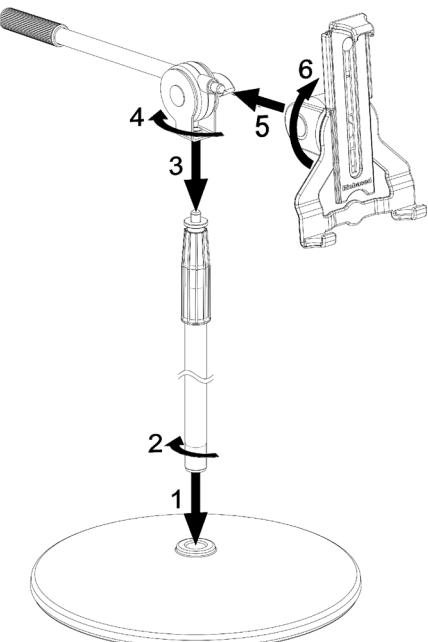
Set the rod combination on the base 1 and screw fully into the base 2.
