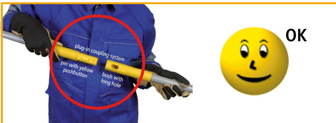
**Figure 8** Single parts with a "YELLOW"- "YELLOW" combination
