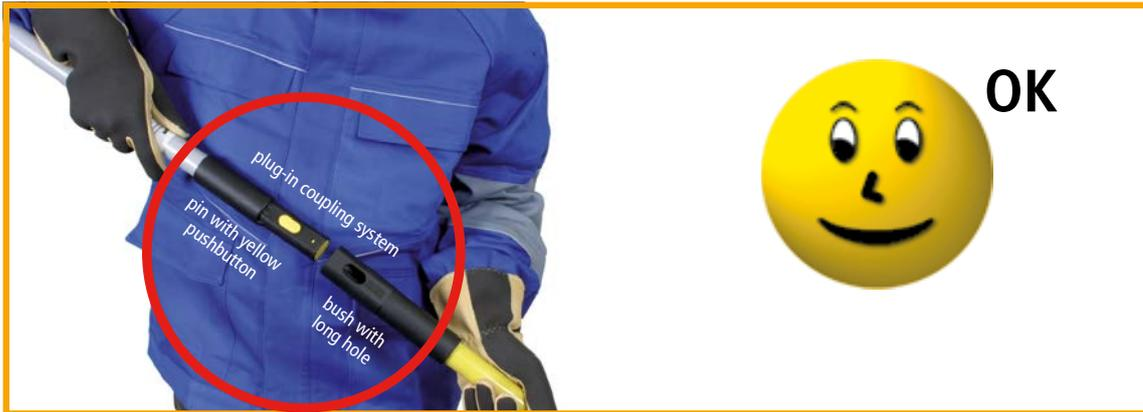
**Figure 9** Single parts with a "BLACK"-"BLACK" combination
