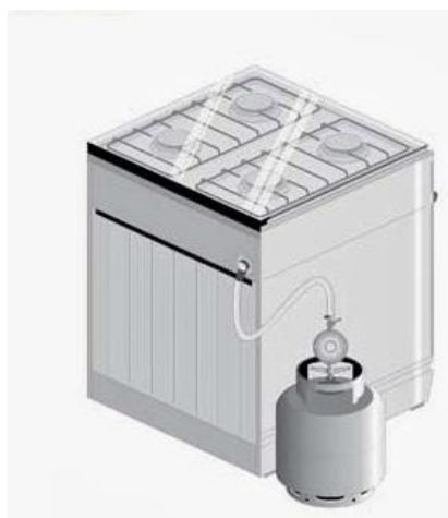
Figure 1 – Typical LPG gas cylinder assembled with a stove in Brazilian residences. [4]
