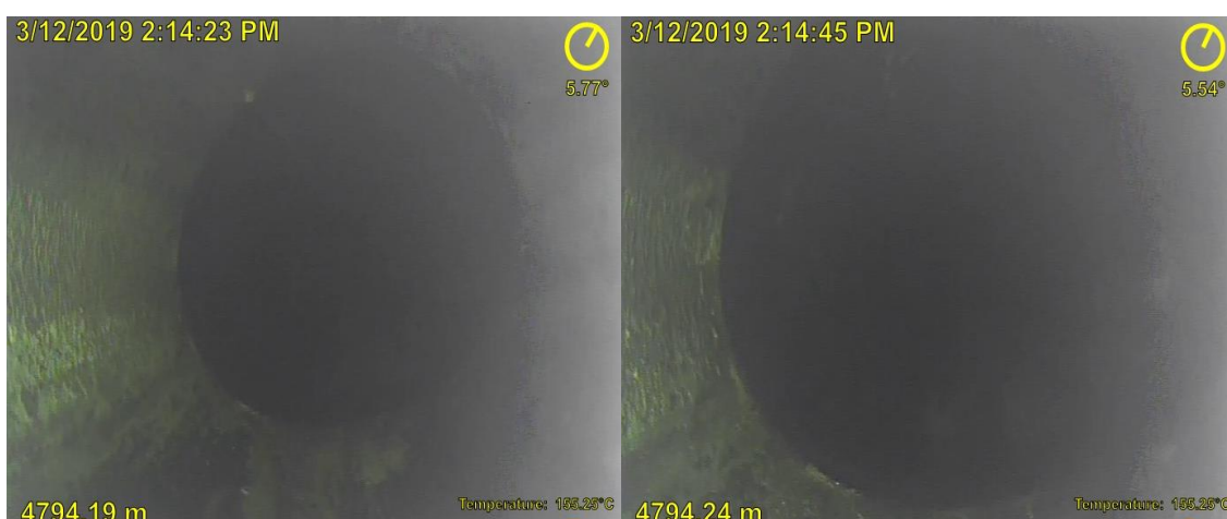
Abbildung 5: 3 ½" Tubing-Shoe (Down - View)
