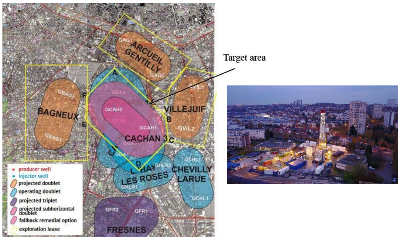
Fig. 4—Paris Southern suburbs: geothermal district heating doublets and triplets locations, and view of the rig in Cachan.
