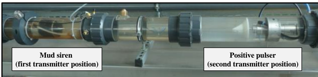
Figure 12: Combination of the Mud Siren and Positive Pulser (Berro and Reich, 2019)
