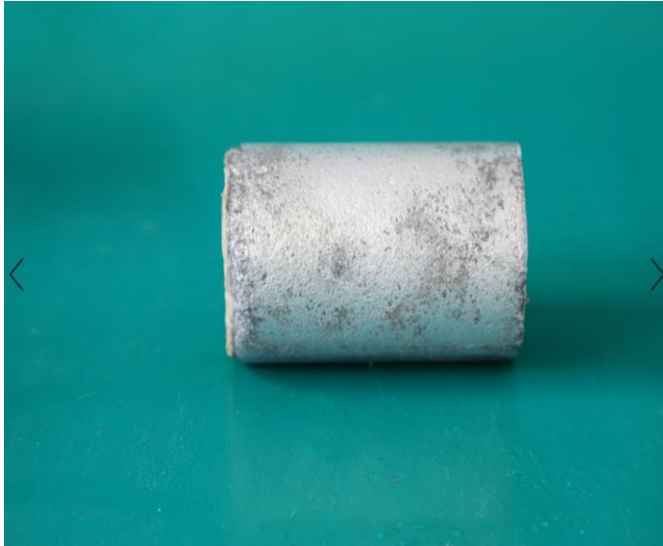
Figure 13: Corrosion effect observed post CO 2 flooding
