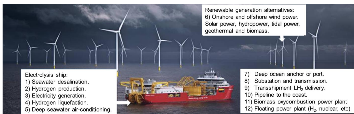
Figure 5: Electrolysis ship components.
