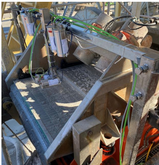
Camera &amp; light setup over a shale shaker
