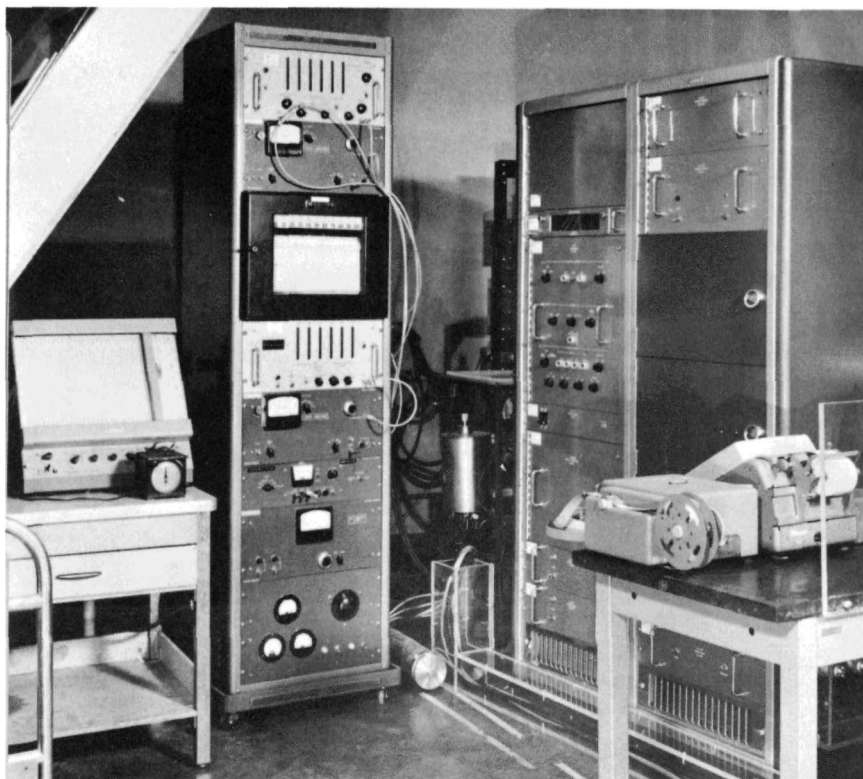
Fig. 6. Part of the Electronics Instruments. Left to right: the X-Y recorder; a console containing the measuring scaler, the amplifier unit (including the rate-meter, the discriminator for the B^{10}F_3 counter, and the DC power supply), Brown recorder, the preset scaler, the amplifier unit for the fission counter, the power supply for the potentiometer and the recorders, the high-voltage power supply for the B^{10}F_3 counter, the power supply for the high-temperature furnace; the automatic control unit.
