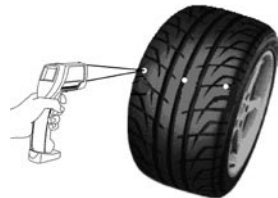
Fig. 8: Measuring Tire Temperatures
