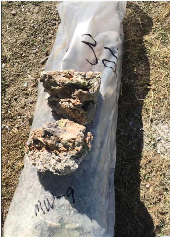
Boring MW-9 fanglomerate from 32 to 34 feet, semi-consolidated, light gray to grayish-green to grayish-maroon silty clayey matrix with angular quartzitic pebble clasts and cobbles
