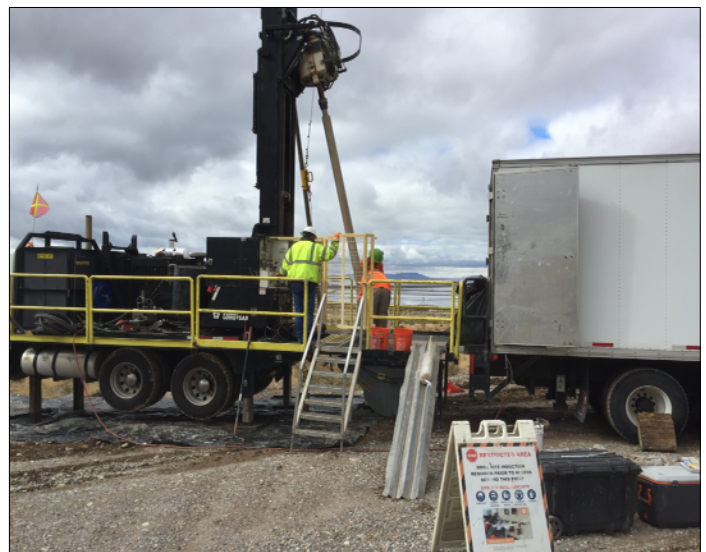
Removing core samples from core barrel
