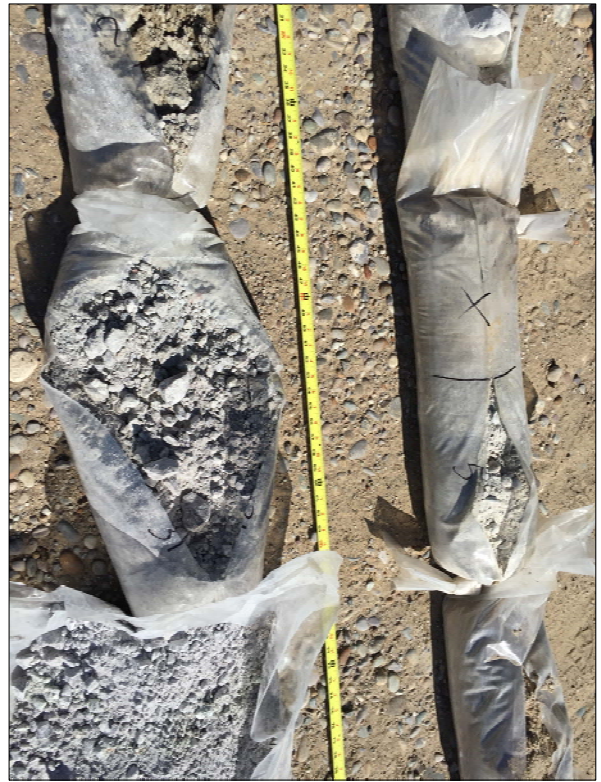
Boring MW-8 fanglomerate showing the abundant light gray silty matrix
