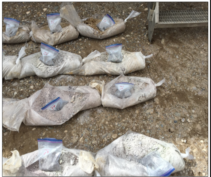
Boring MW-7 Lake Bonneville and fanglomerate samples laid out sequentially
