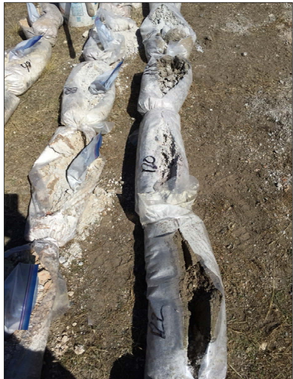
Boring MW-9 fanglomerate cores showing variability of fanglomerate in core from 40 to 122 feet, highlighting dark brown silty sand and gravel layer at 121 feet.
