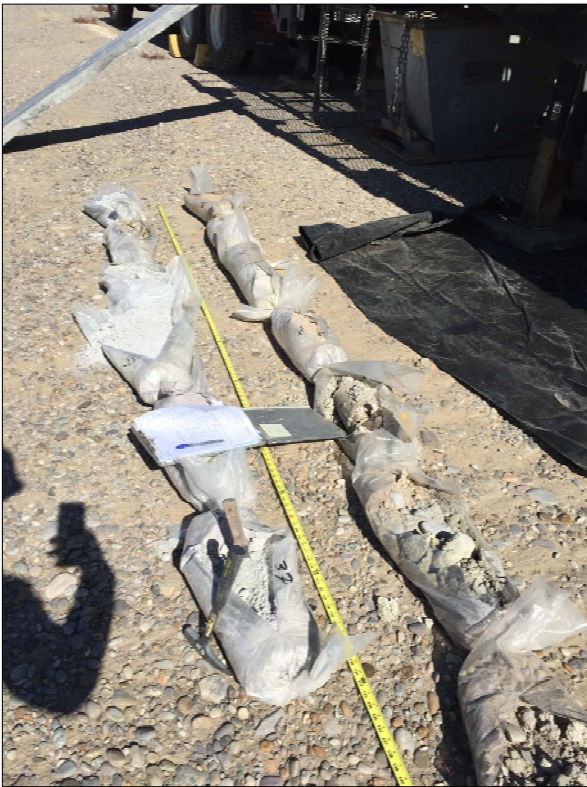
Boring MW-8 Lake Bonneville from 0 to 12 feet and fanglomerate from 32 to 37 feet, semi-consolidated, light gray silty clayey matrix with angular quartzitic pebble clasts and cobbles
