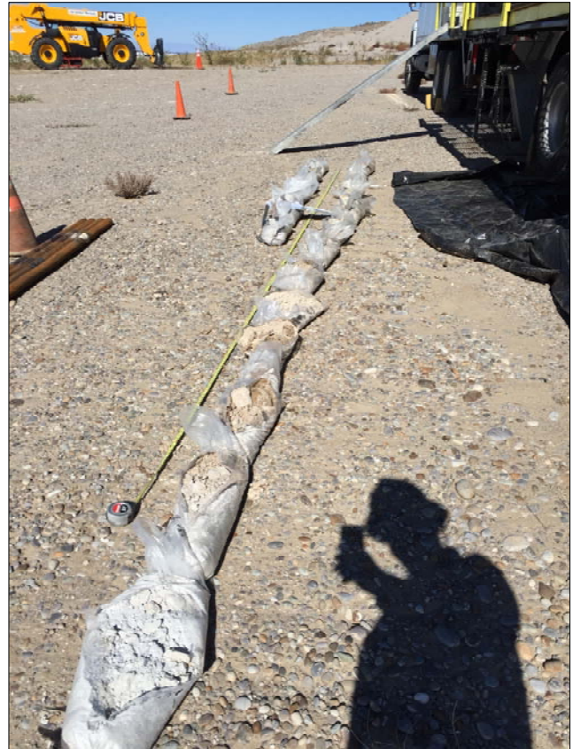
Boring MW-8 fanglomerate contact with Bonneville sediments at 30 feet
