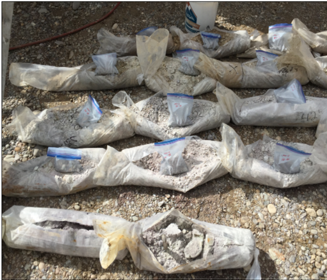
Boring MW-7, including sections of Lake Bonneville sediments from 0 to 24 feet and fanglomerate sections from 24 to 75 feet, semi-consolidated, light gray silty clayey matrix with angular quartzitic pebble clasts
