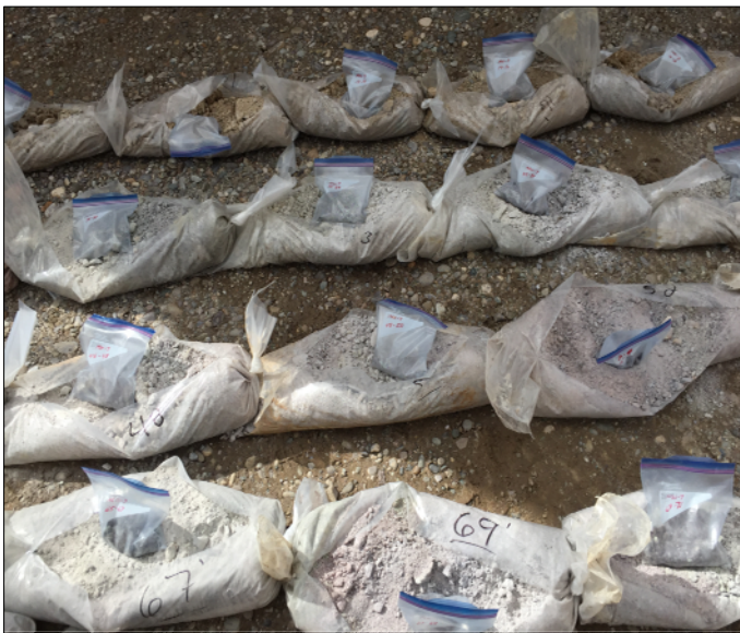
Boring MW-7 showing sections of Bonneville sediments 12 to 21 feet and white to gray silty fanglomerate in sections from 31 to 71 feet
