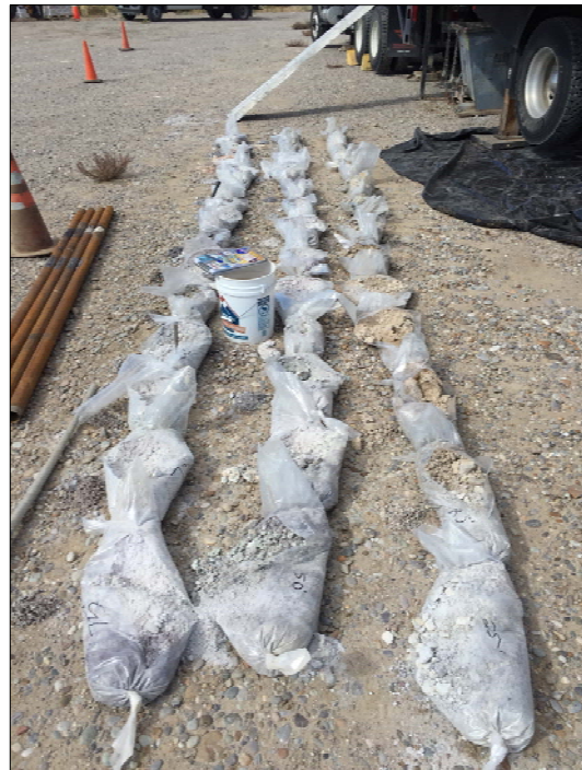
Boring MW-8 samples laid out sequentially from 0 to 75 feet.
