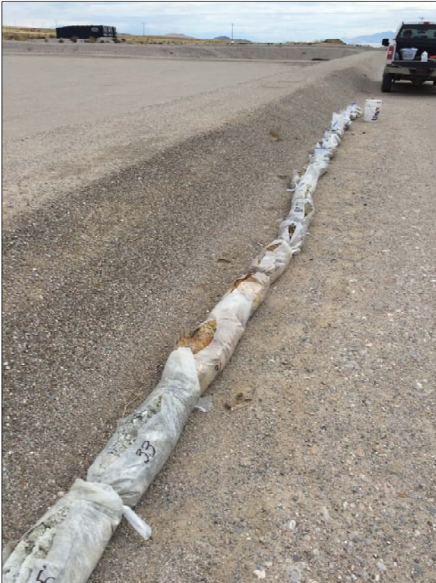
Boring MW-6, sections of Lake Bonneville sediments from 0 to 29 feet with contact with fanglomerate and sections to 35 feet, semi-consolidated, light gray silty clayey matrix with angular quartzitic pebble clasts
