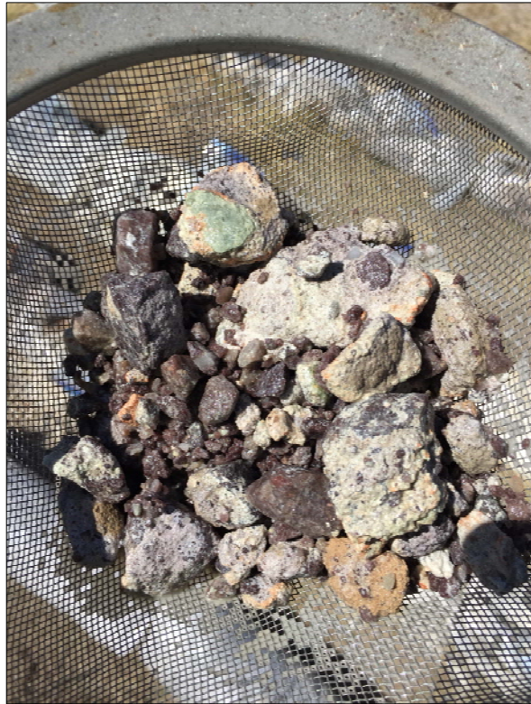
Boring MW-9 fanglomerate with fines washed from sample, light gray to grayish-green to grayish-maroon clay and angular quartzitic pebble clasts
