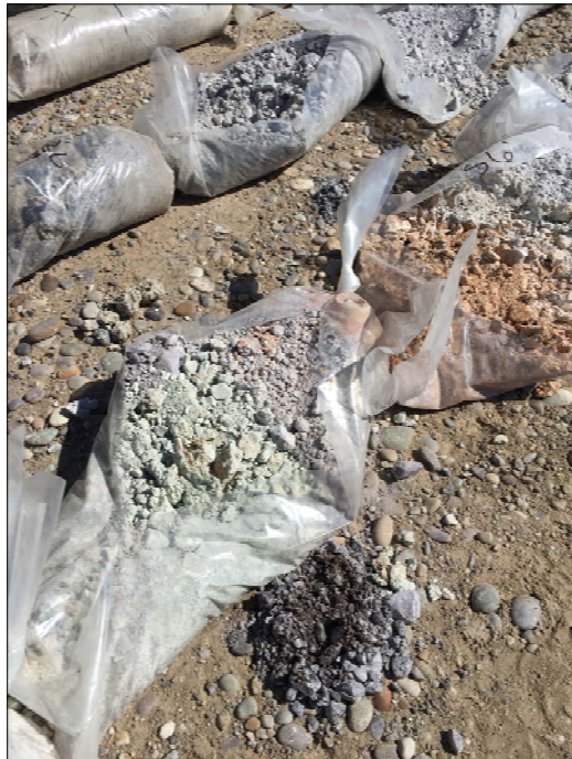
Boring MW-8 fanglomerate showing the variation in color including orange-white clayey gravel with orange-red hematite mottling, non reactive
