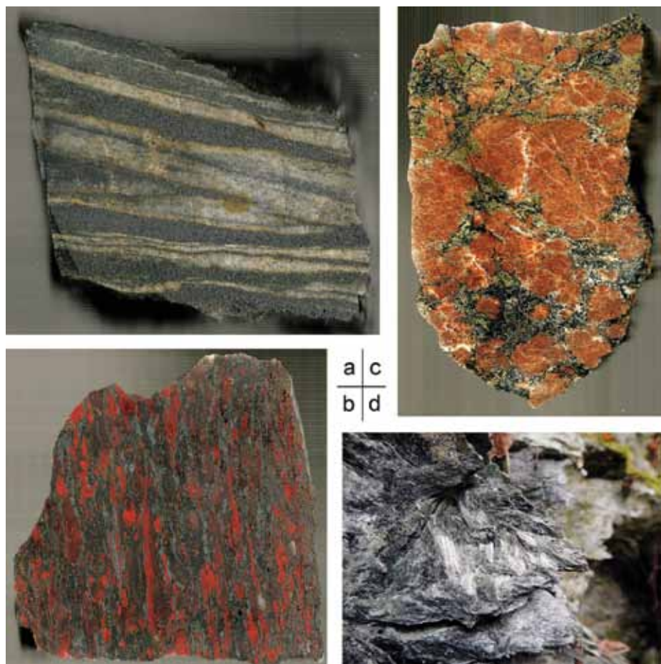
Photos illustrating (a) BIF from Mnisske jamy (Jeseniky Mt.), (b) Jasper like ore, (c) Spessartine rich skarn, (d) Talc from Zadni Hutisko.
