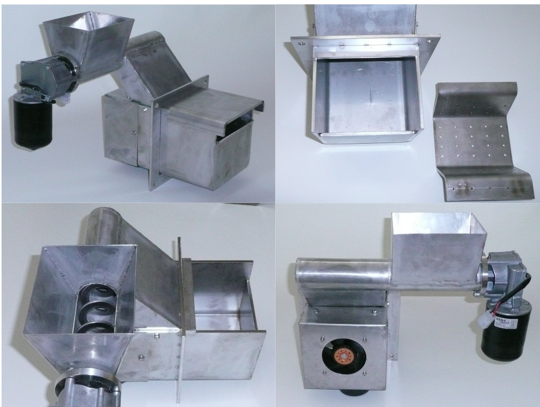
Fig: 6-5. Fabricated shell burner.
