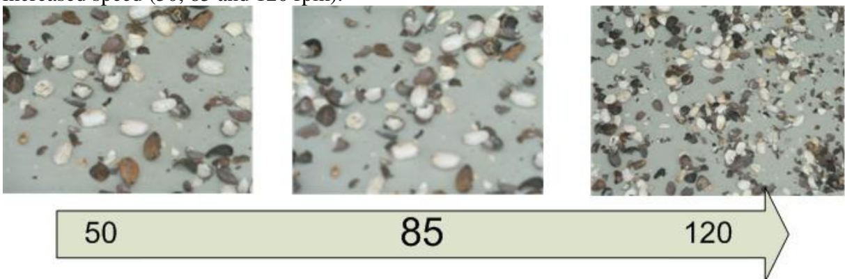
Fig. 1 – 17 Deshelled J. curcas seeds with three different levels of rotational speed J. curcas deshelling efficiency was reduced with the increase of rotational speed from 50 to 120 rpm, more broken kernels were found at higher velocity of rotating cylinder whereas at lower velocity the deshelled kernels were less broken.
