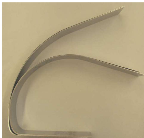
Figure 1.2: Specimens of the sheet metal DP600 with thicknesses of 1mm and 2mm after being subject to bending-tension shown in Figure 1.1 (Kleiner et al., 2005). After the bending-tension test is carried out, the specimens are released from the clamps and spring back into their final forms shown here.
