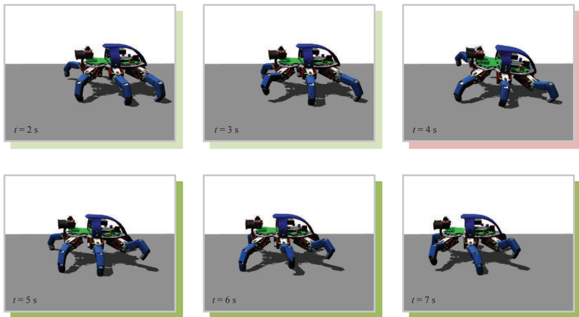
Figure C.2: Simulation of the DLR Crawler experiencing the loss of its left hind leg (L3); light green frames: the robot is fully functional, red frame: the left front leg is lost (i. e. lifted and hold in this position), green frames: the robot instantaneously adapts its gait, shifts its COG away from L1 and increases its joint stiffness settings
