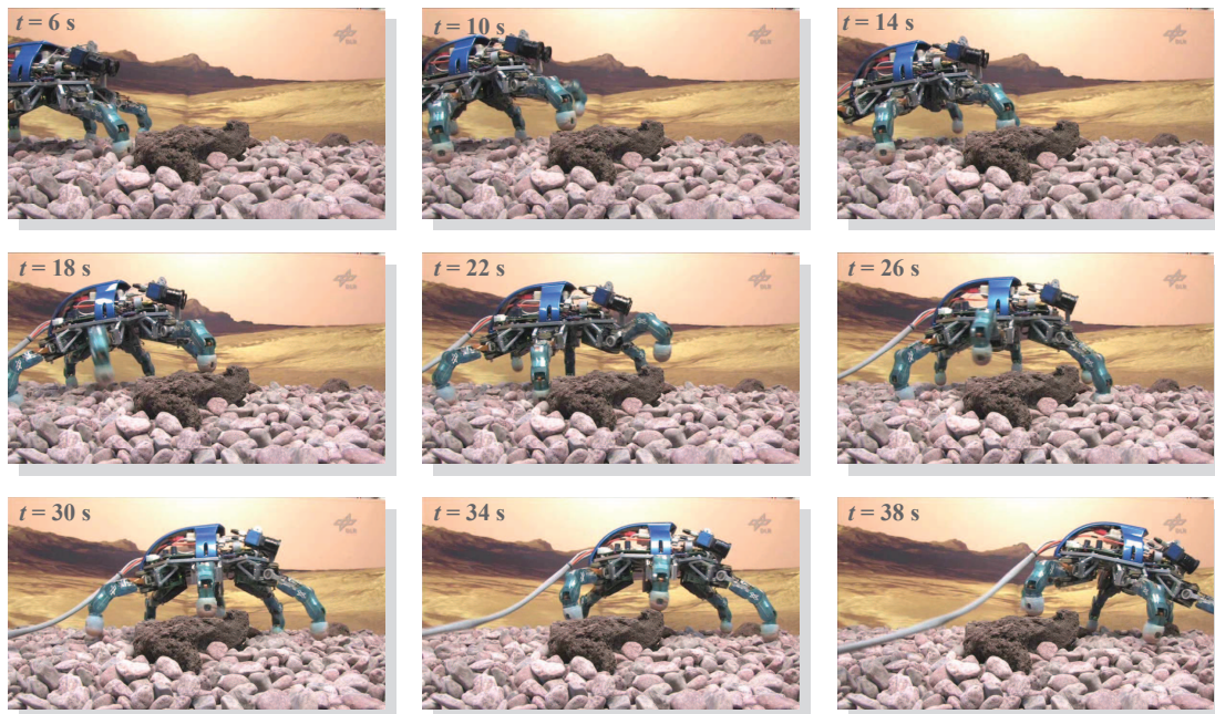
Figure 4.25: The DLR Crawler crosses stones within the indoor gravel testbed
