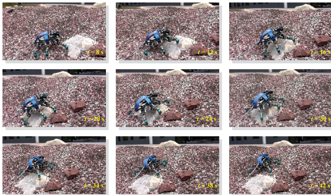
Figure 4.27: The DLR Crawler climbs a 30^\circ slope within the DLR outdoor testbed
