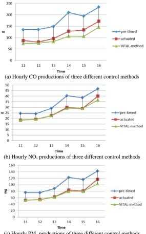
(c) Hourly PM<sub>x</sub> productions of three different control methodsFig. 8. Comparison of the simulated emissions.
