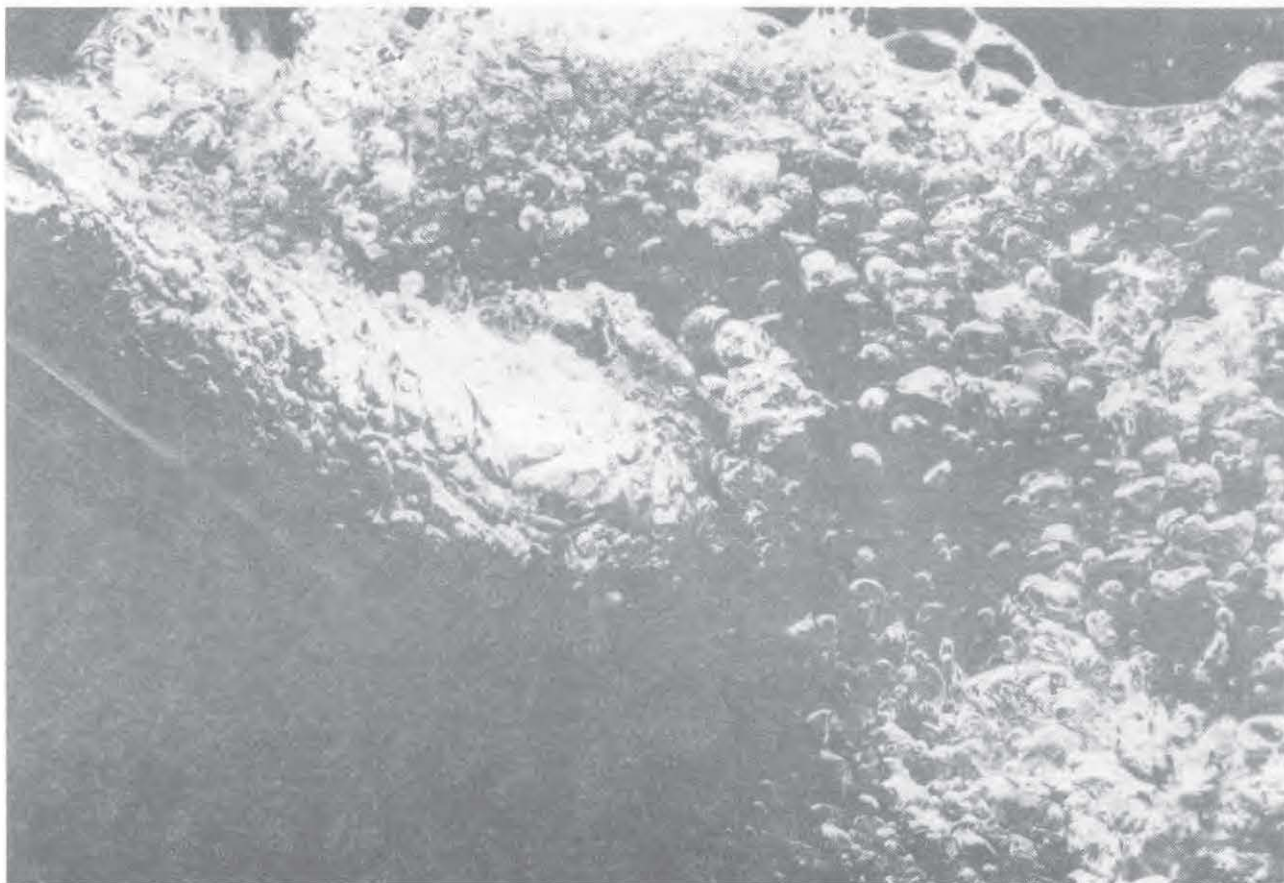
Fig. 1.5: Air entrainment in a supported inclined jet by vortices with axes perpendicular to the flow direction (a) overall view (Photo: I. Wood, 1984) (b) close-up of foam layer and vortex (Photo: N. Thomas in Goldring et al, 1980)
