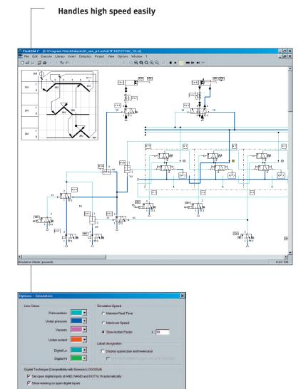
The circuit model on the left contains more than 5,200 variables, of which 1,500 are continually changing. In a simulation, an integration procedure has to calculate 110 status variables (pressure, position, speed, etc.) at an accuracy between 1 in  $10^6$  to  $10^9$ , which must be maintained in relative and absolute terms.
