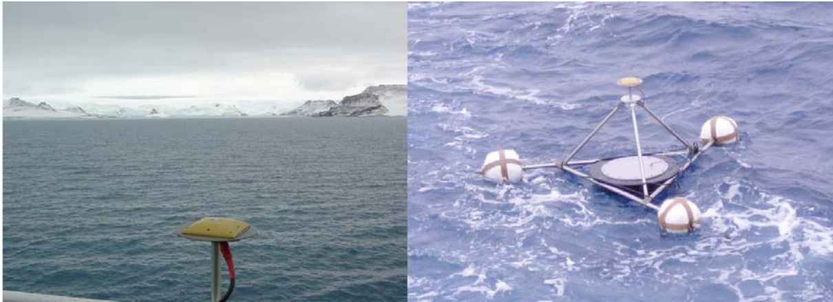
Fig. 8.1: View of the bow GPS antenna Fig. 8.2: View of wave-rider GPS buoy
