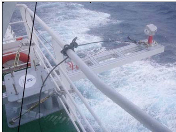
Fig. 8.3: View of the Optiwave radar altimeter
