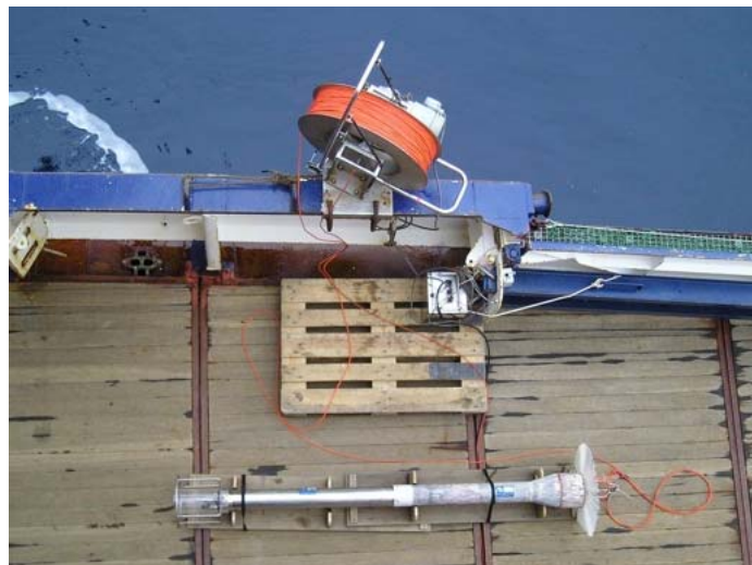
Fig. 3.8.1: TurboMAP microstructure profiler
