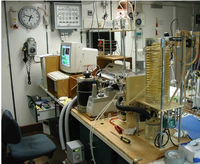
Fig. 5.1: Integrated TA and TCO 2 titration system on board Polarstern
