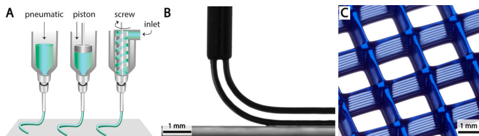
Figure 3. Robotic dispensing. (A) Schematic drawing of robotic dispensing showing the different mechanisms of ejection. Reprinted in part with permission from ref 27. Copyright 2013 John Wiley and Sons. (B) Magnified view showing material dispensing from the needle and collection onto a substrate. (C) Stereomicroscopic image of a printed Pluronic F127 construct.
