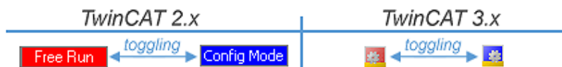
Fig. 131: Displaying of “Free Run” and “Config Mode” toggling right below in the status bar
