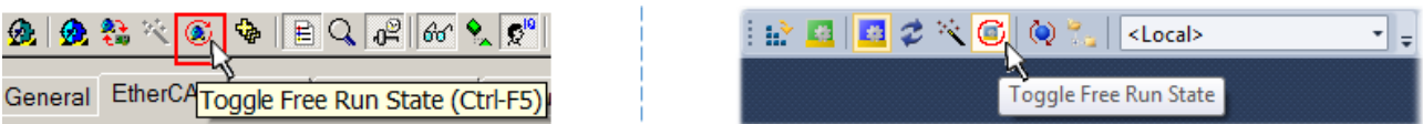
Fig. 132: TwinCAT can also be switched to this state by using a button (left: TwinCAT 2; right: TwinCAT 3)
