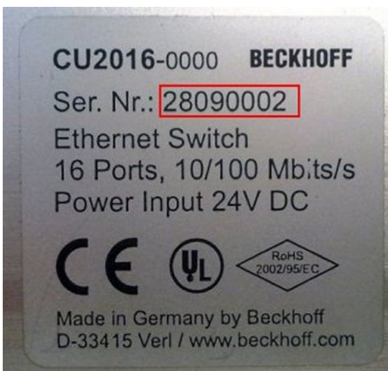
Fig. 3: CU2016 switch with serial/ batch number
