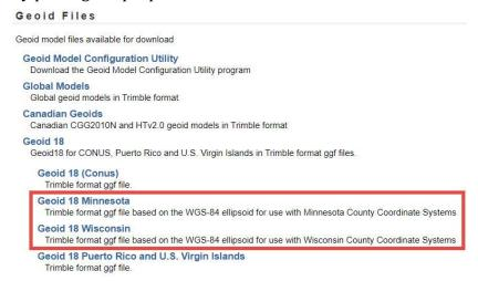
Once downloaded, you need to put the \*.ggf file in the proper folder for your Coordinate System Manger is located and referencing. By default this is C:/Program Data/Trimble/GeoData.
