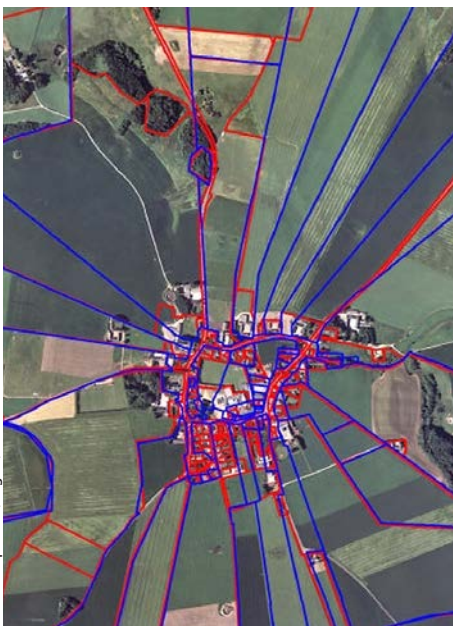
◀ Fig. 5: Example of star allotment of the village of Vellev, Mid-Jutland. Blue lines represent cadastral boundaries as of 1880, red lines represent boundaries as of 2000. Note that the later subdivisions occur within the village's built-up area only, an outcome of the well-functioning spatial planning.
