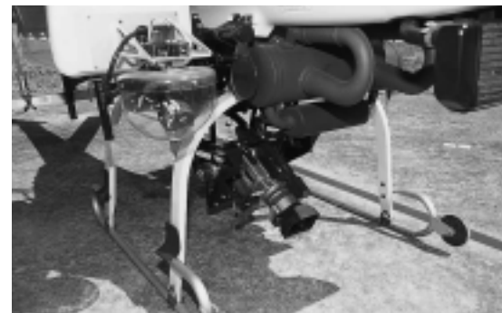
The camera mount on the "Aerial RMAX"
