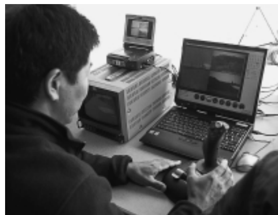
Images from the Autonomous Flight RMAX's CCD camera appear real-time on the PC screen so the operator feels like he is in the pilot's seat
