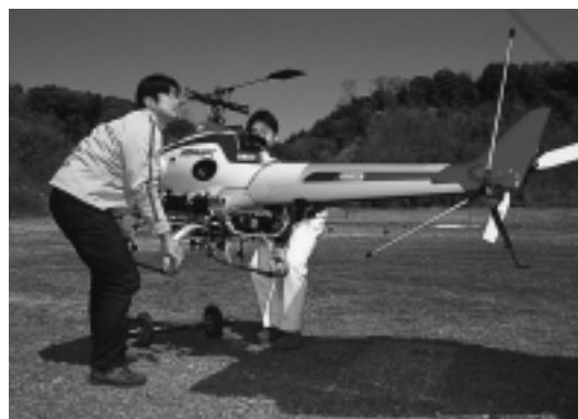
The RMAX is designed to be carried by two people for ease of use on the farm
