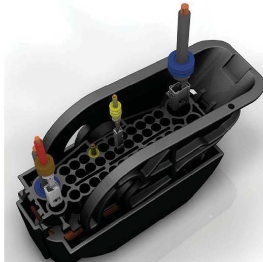
Fig. 14: 38-way connector, equipping with terminals Abb. 14: Kabelbaumstecker 38-polig, Kontaktbestückung
