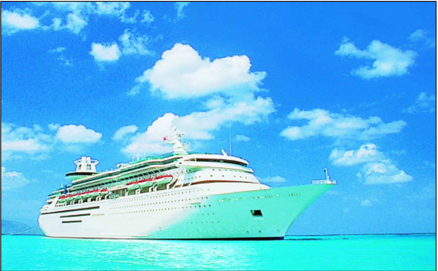
The cruise ship Sovereign of the Seas measures 73,192 gross tonnage, but displaces only 34,300 long tons in a fully loaded condition. Courtesy Royal Caribbean International.
