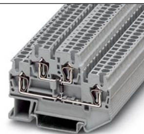
26 A, double-level diode terminal block, 1N 4007 (1300 V/0.5 A)
