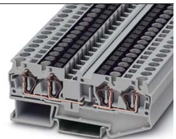
37 A, feed-through terminal block, 4 connections, with interrupted current bar
