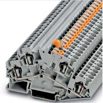
4 (6) mm 2 , 34 A, double-level knife disconnect terminal block
