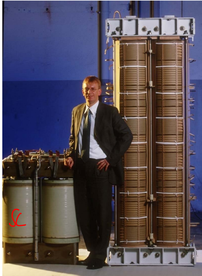
HTS-Train transformer left Normal train transformer right
