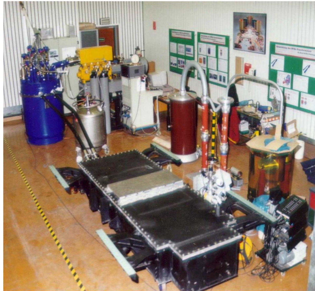
HTS-Transformer in test field
