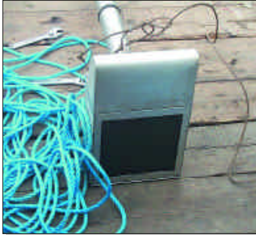
Figure 2 Parametric transducer in a stream-lined hull ready to mount over the side of the vessel
