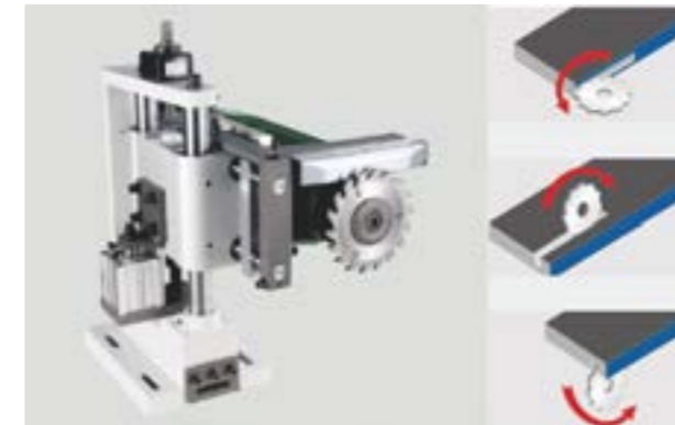
Hogging Available with multi hogging directions.
