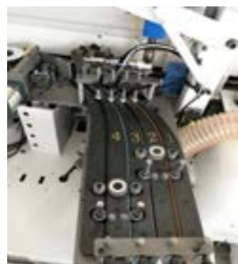
4 Positions servo edge feeding (Option)
