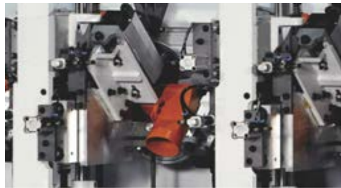
Pneumatic Control System Automatically change between 4 different kinds of edge thickness.
