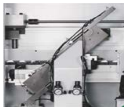
Tilting End Cutting
