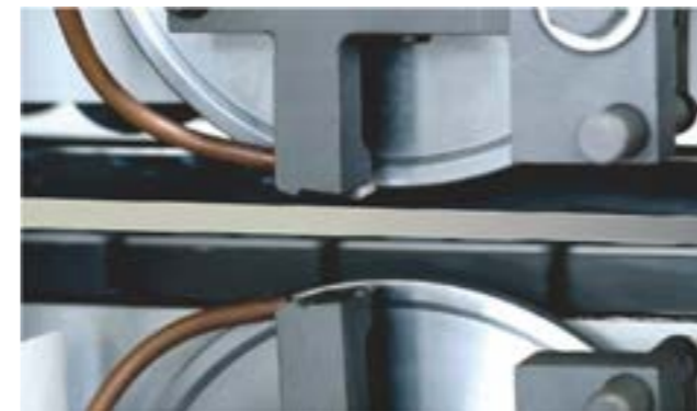
Flat scraping mechanism Scrapping off the visuable glue line,to make surface more smooth beautiful.
