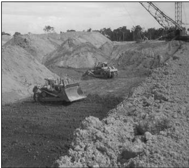
Figure 3: Strip mining at Trombetas mine. Bulldozers ripping lateritic crust [SP2-2000].
