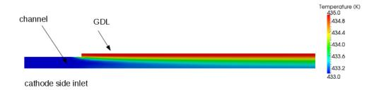
Figure 3.45: Temperature profile on the cross-sectional plane B (only the first 25 mm are showed).
